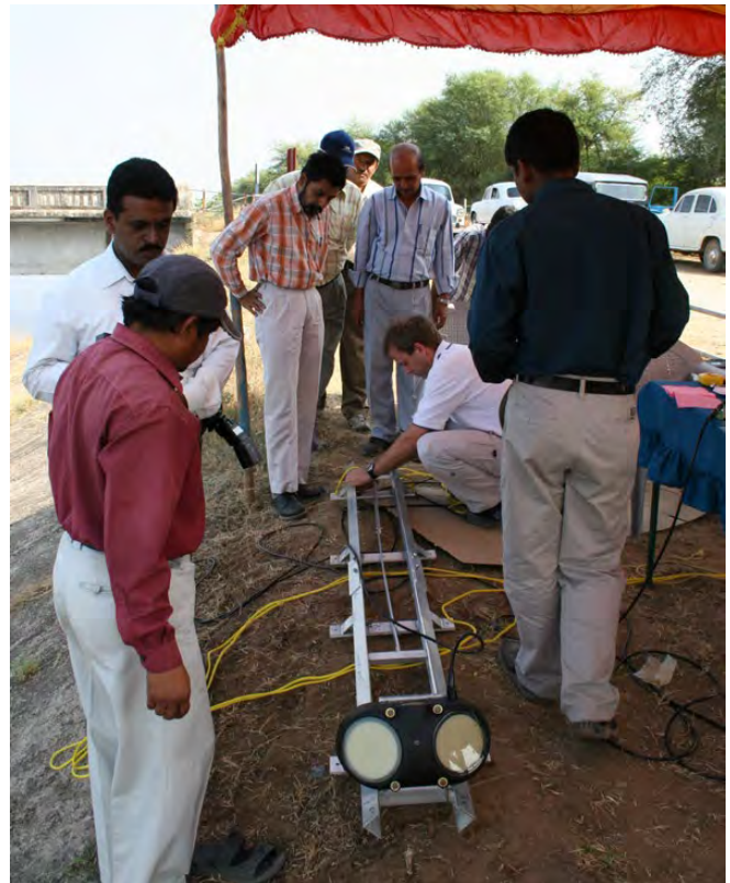
Installation of a Argonaut-SL500 ("side-looking") into the Narmada canal.
